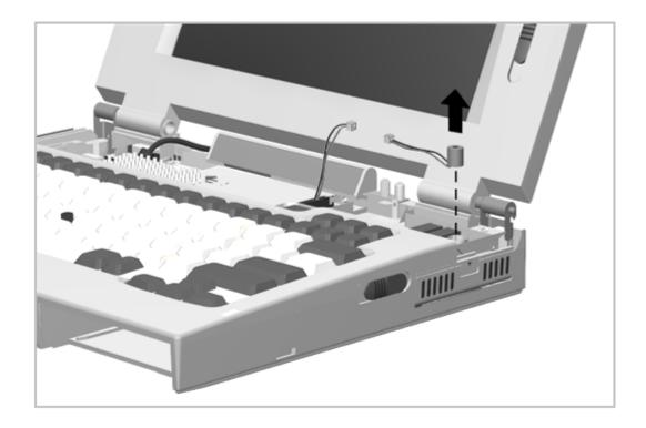
Figure 5-27. Removing the Microphone
